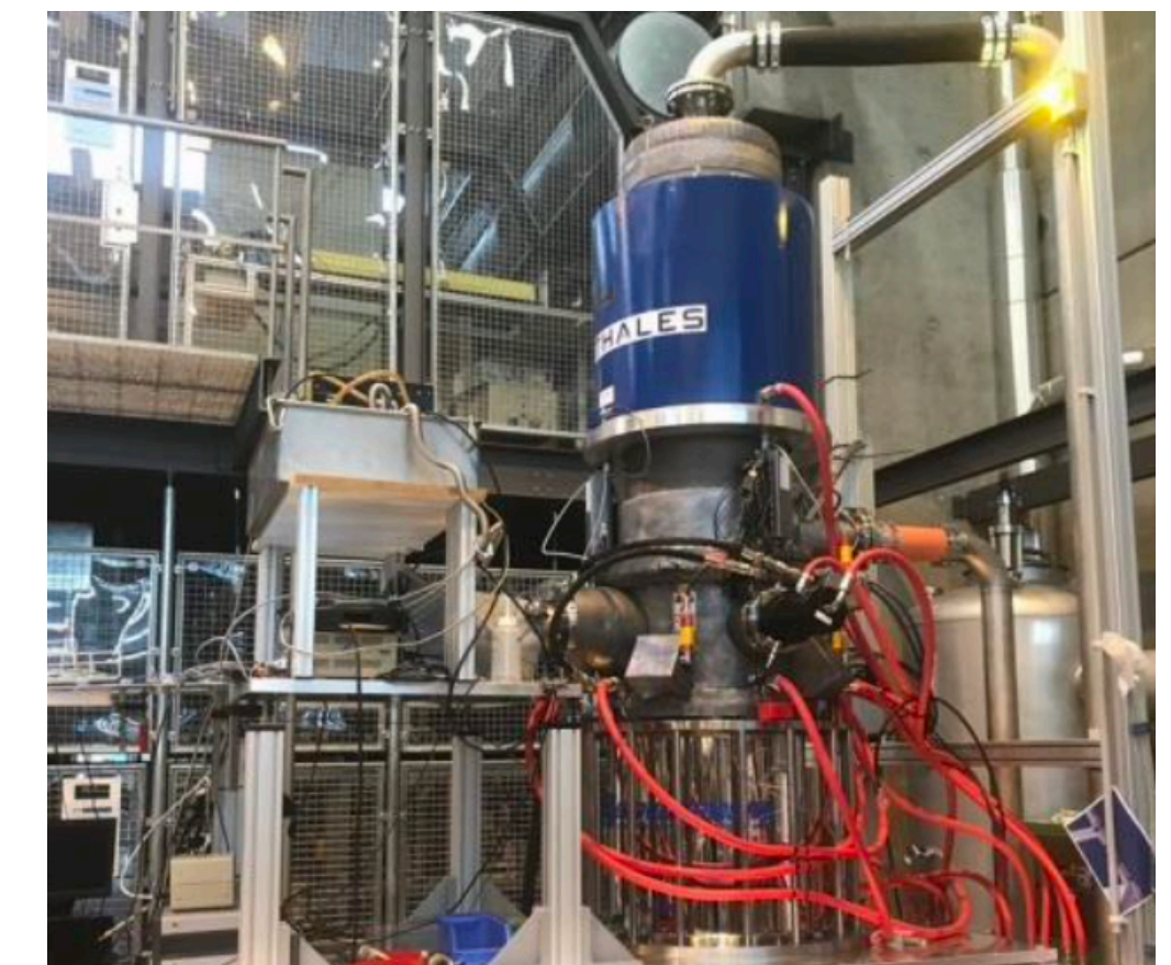
TCV gyrotron for ECRH
